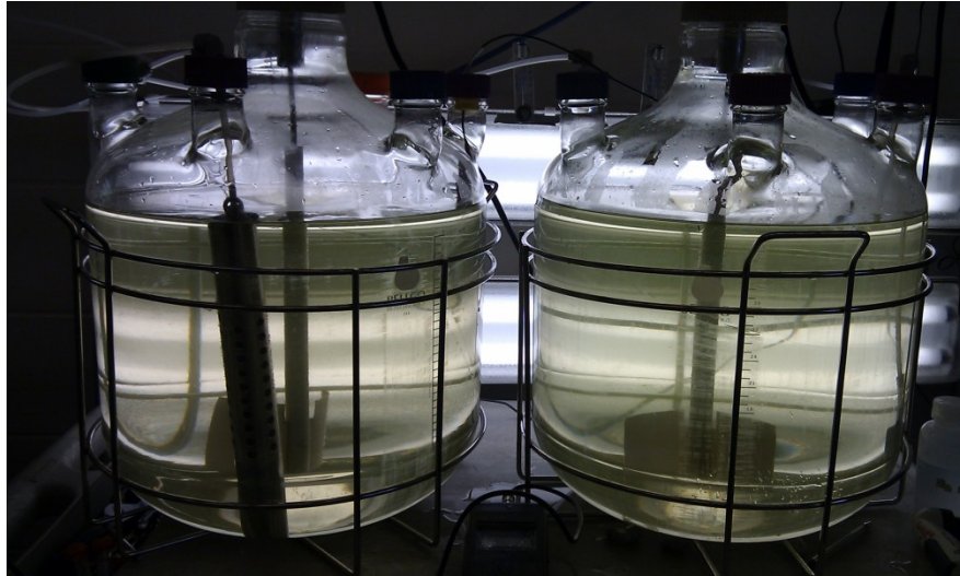
Figure 3-1: Bellco jars set-up with HFM (L) and diffuser (R). Flowmeters and gas flow sensor in background.
