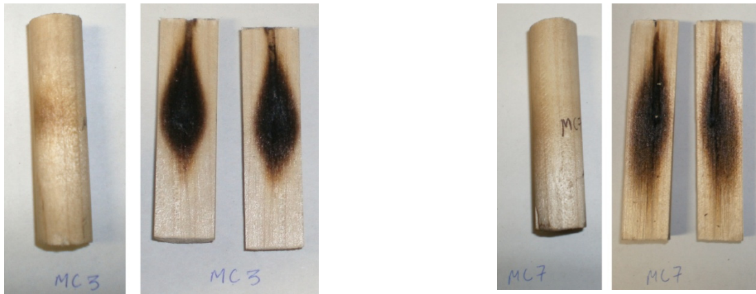
Figure 4-15: Microwave Torrefaction of a 19 mm diameter poplar wood (5.4% moisture) at 280 C, (a) for 5 minutes, Mass yield obtained 94%. (b) for 10 minutes, Mass yield obtained 91.9%. The figure shows photograph the exterior of the cylinder after torrefaction and after splitting
