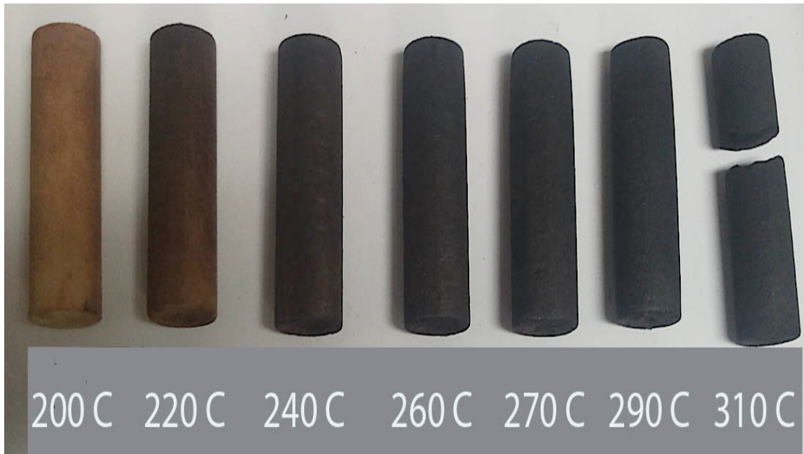
Figure 5-2: Picture of Oak cylinders (22mmx64mm) torrefied at various temperatures for a 60 minutes reaction time.
