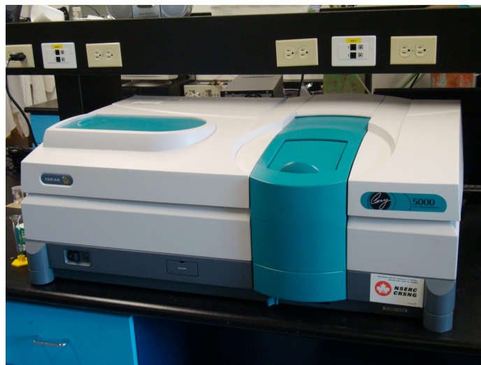
(b) Varian Cary 5000 Spectrometer. The optics and loading stage are installed in the chamber of the spectrometer. They are not visible on the picture.
