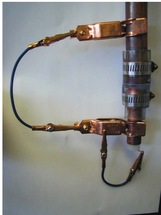
Figure 6.2 Picture of simulated 40:60 Pb/Sn soldered joint.
