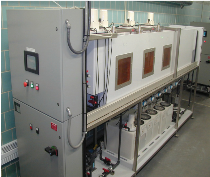
Figure 3.2 Photo of pilot plant coagulation, flocculation and sedimentation skid.
