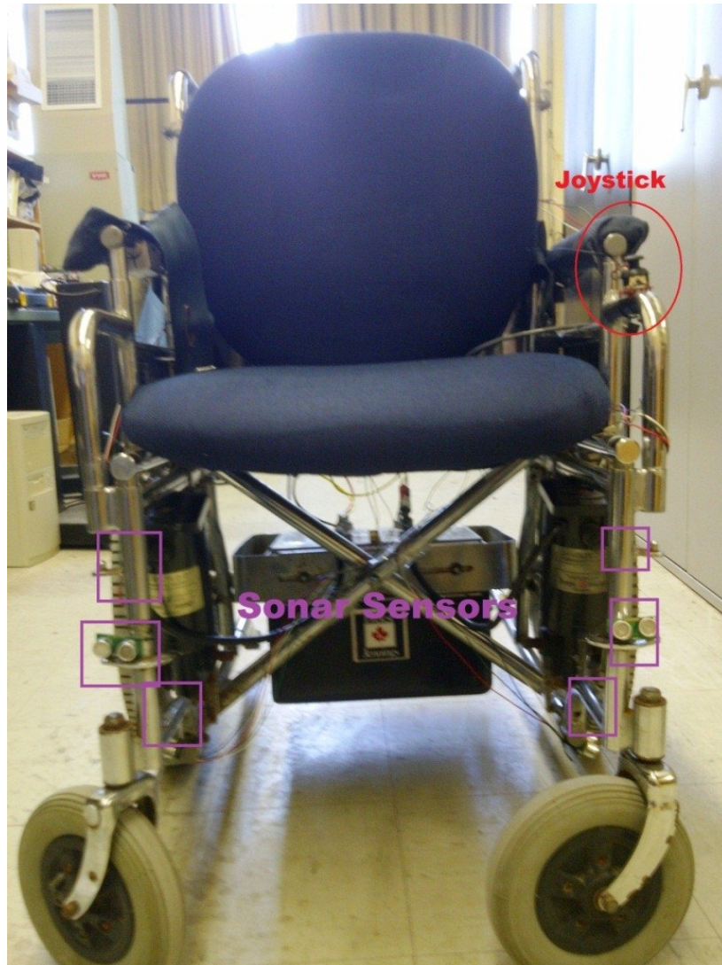
Figure 6.2: The smart wheelchair sonar sensors and joystick implementation
