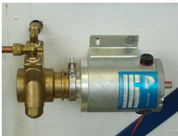
Figure 57 The glycol circulation pump.
