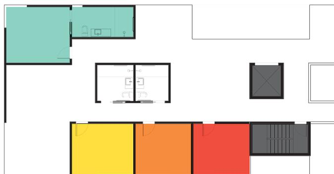
Figure 52: Partial upper floor plan, accommodating an elderly person with a live-in caregiver and a palliative care facility, where residents have a private room in addition to communal facilities.
