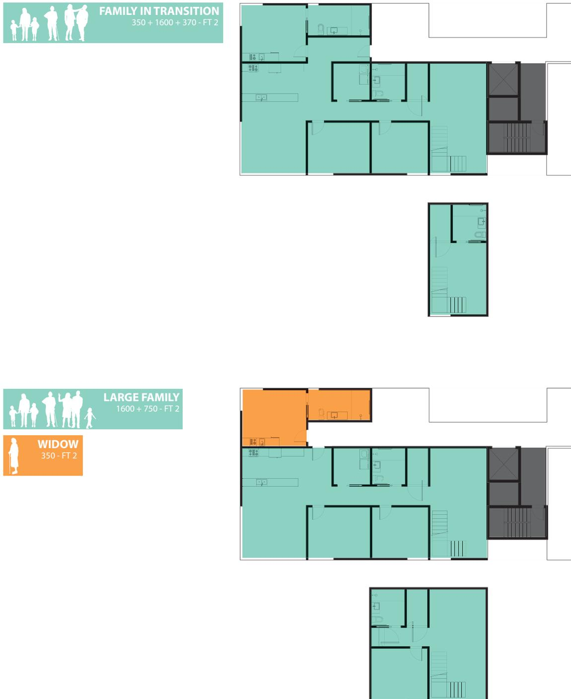
Figure 50: Partial upper floor plan, demonstrating how a single unit can grow and accommodate large families, allowing an extended family to exist within the same apartment while keeping their own space.
