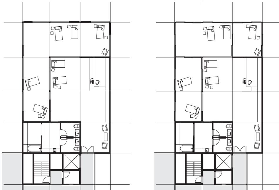
Figure 28: Partial first floor plans demonstrating how the assisted living facility is able to open up through the use of a double facade of sliding panels. The interior space is also able to divide in order to provide different amounts of privacy and attention.
