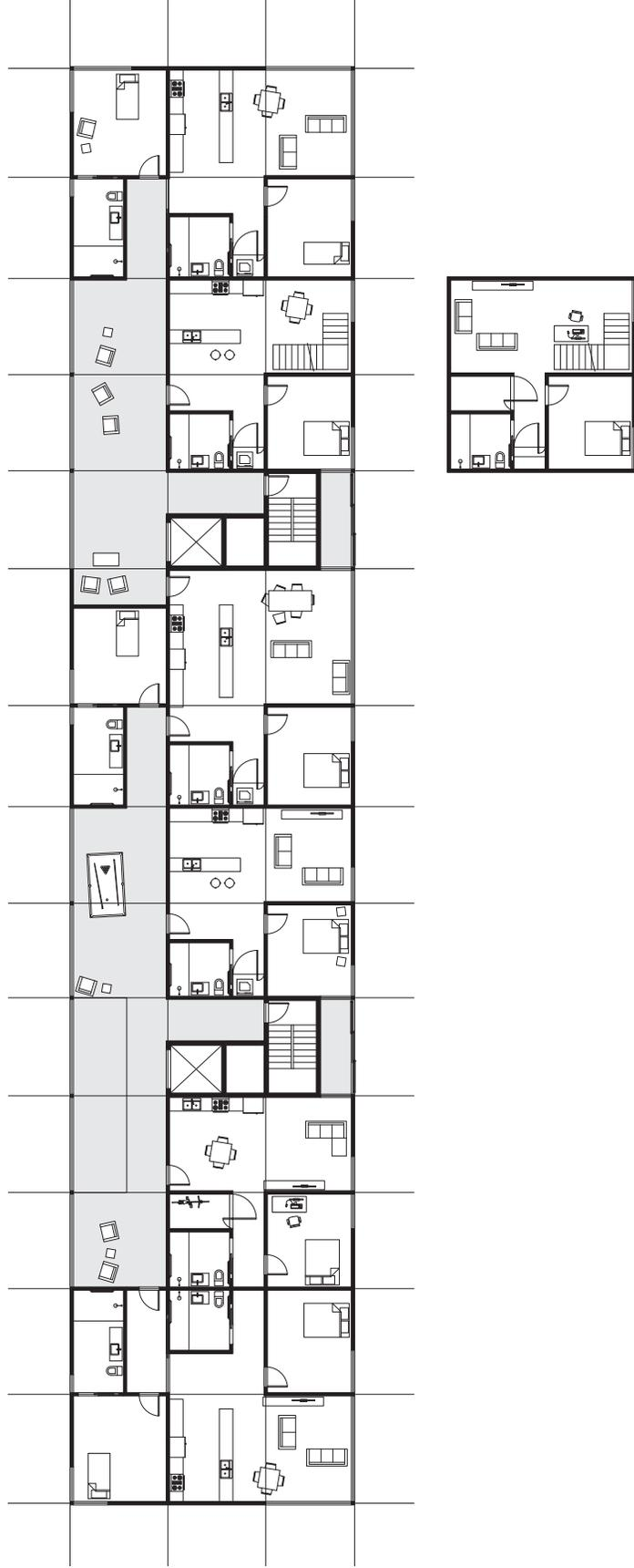
Figure 36: Typical floor plan. Variation 3: small apartments.
