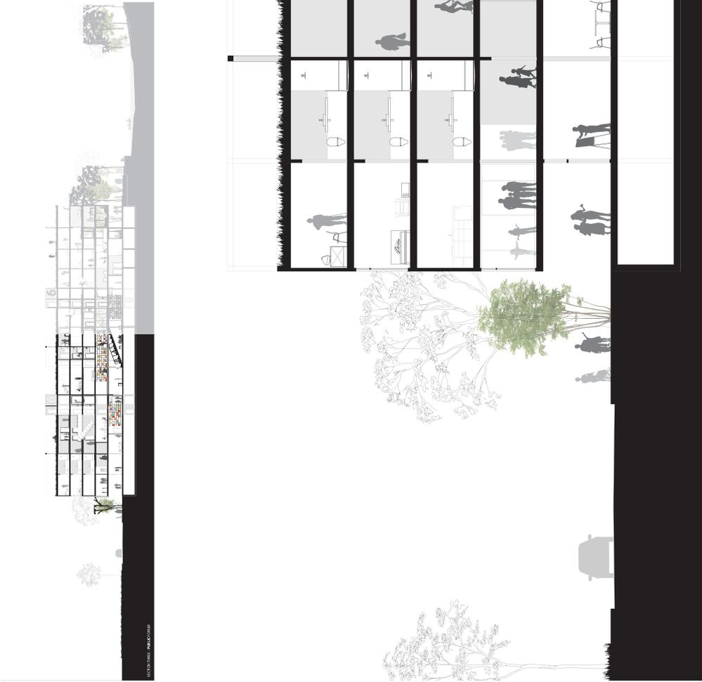
Figure 29: Cross-section (from left to right), showing Eriton Street, the artist studio, reception, and the event space on the ground floor, with the day-care and sun room on the first floor.
