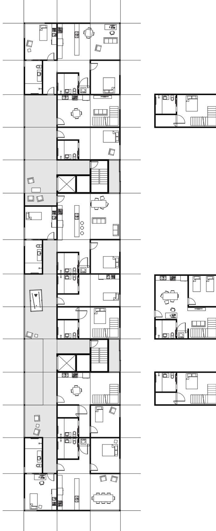
Figure 35: Typical upper floor plan. Variation 2: various apartments.
