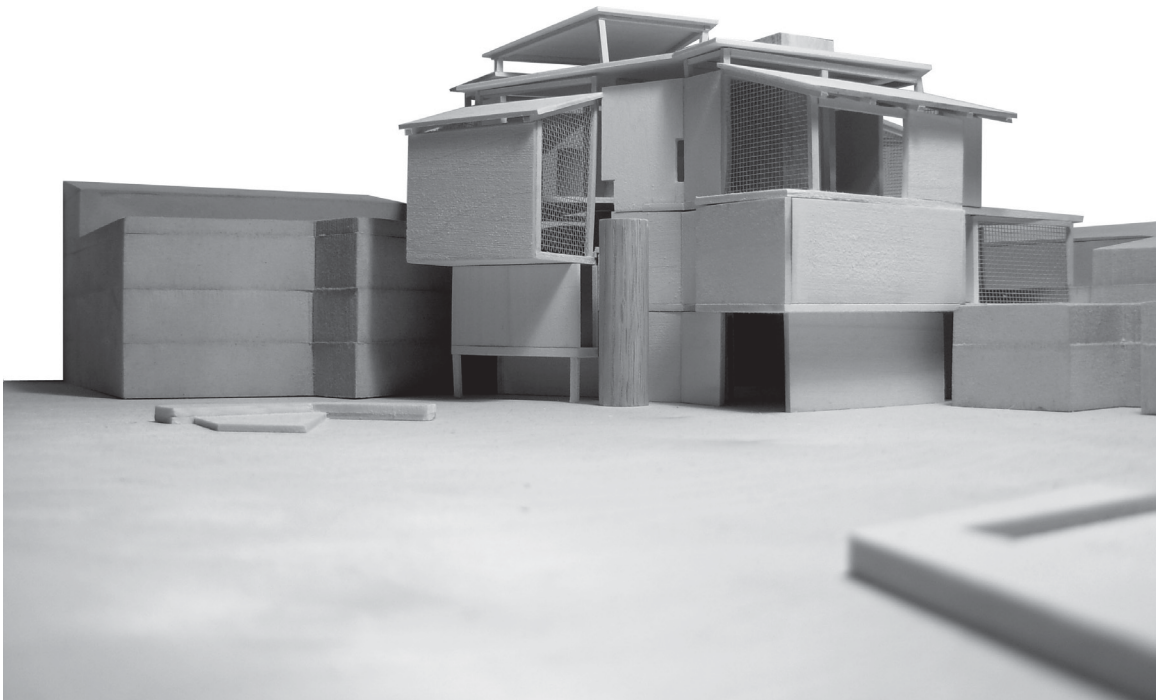
Final Model. Windows along the exterior facade are small allowing light to penetrate and highlight specific spaces, while screened walls allow diffused light that penetrates deep into the building.
