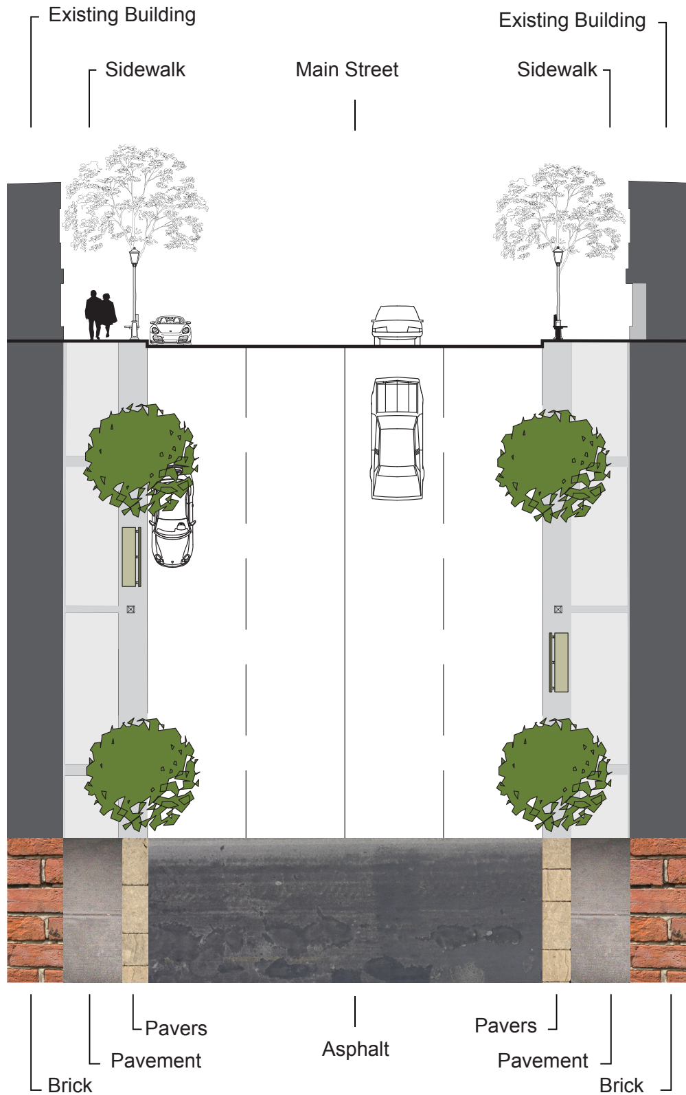
Main Street Typology. Diagram showing the relationship between the street, sidewalk and storefront.
