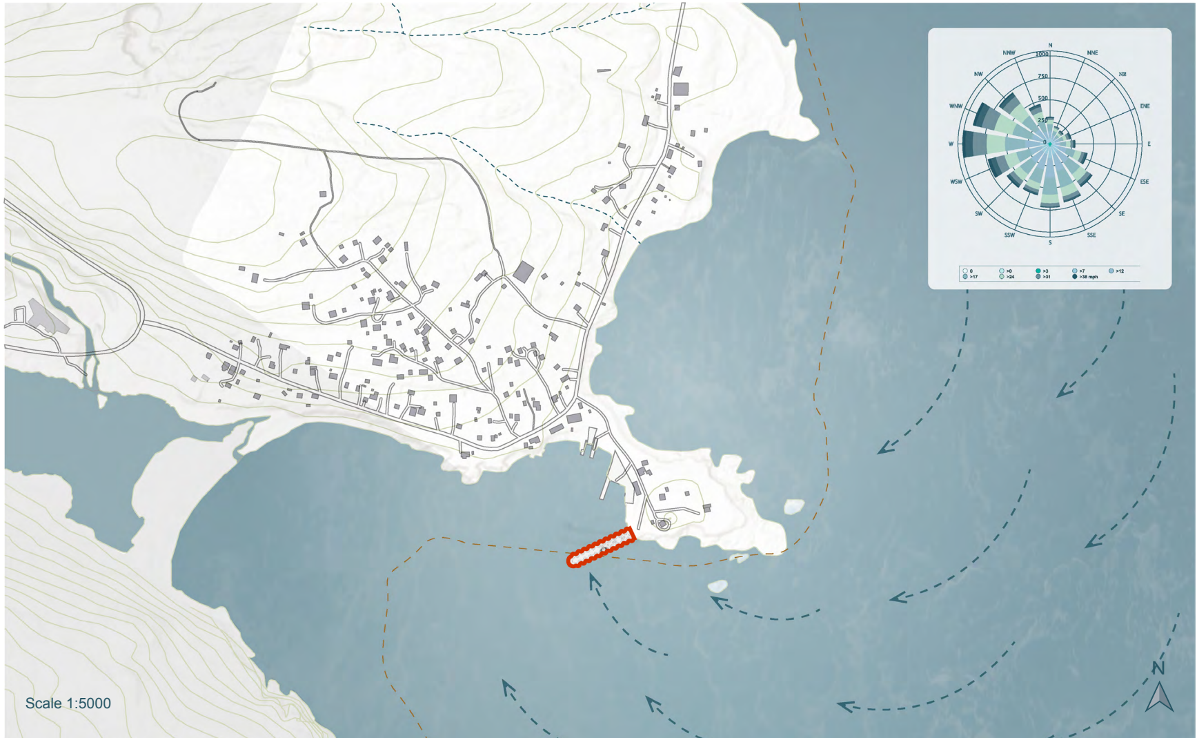
Neil's Harbour regional context map indicating the proposed inhabitable breakwater system, prevailing winds and predominate wave action. (Data from Nova Scotia Open Data).
