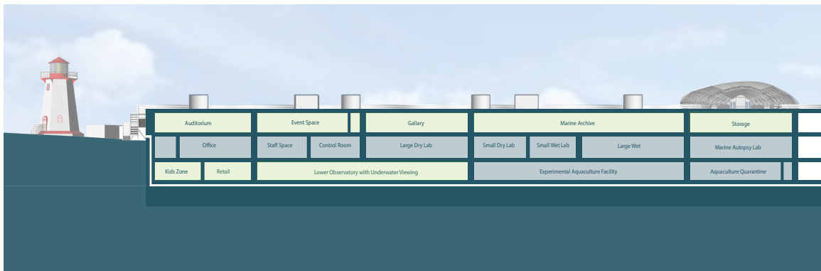
Preliminary longitudinal section indicating the utilization of space and approach to dividing public (green) versus private (blue) program within the inhabitable breakwater.
