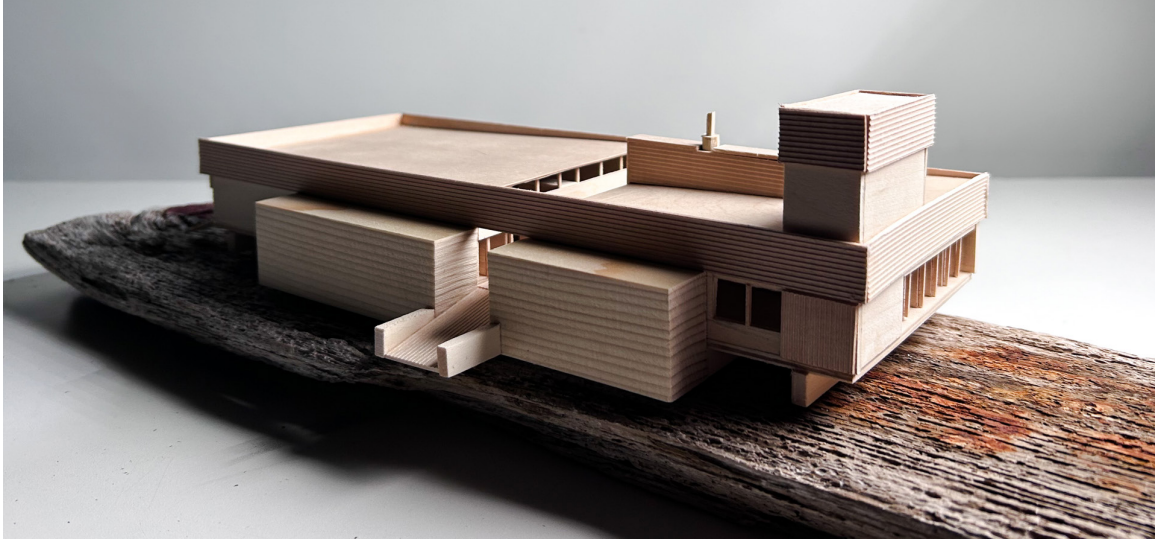
The building's "rocks" sit at the entrance of the building for people to seek refuge behind. These concrete boxes support the fins which the building sits upon.
