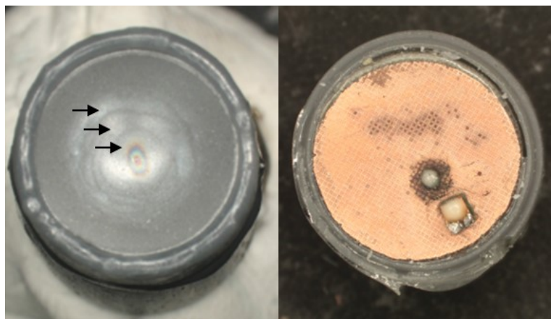
Figure 4.9: Examples of transducer failures, Parylene delamination (left) and electrode failure (right).
