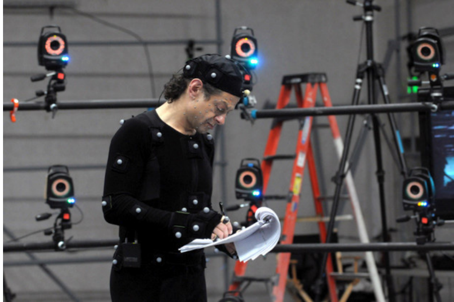
Figure 4 Retroreflective passive marker-based motion capture system used to track movement during a filming process.
