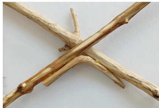
Reinforcing a ridge connection using the concepts of a 'ship's knee'.
