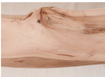
Where the ring pattern breaks and there is grain moving mostly horizontal is continuous tangential grain.
