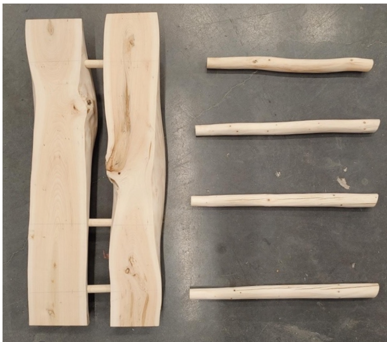
The bench components. On the left the two curved members fastened by machined dowels. On the right are the four legs cut to length and sanded.
