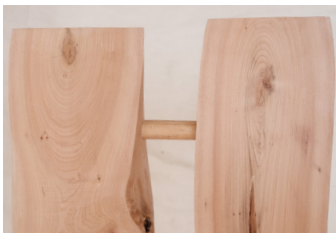
The ring grain pattern shows where grain is exiting the wood, this is the end grain.
