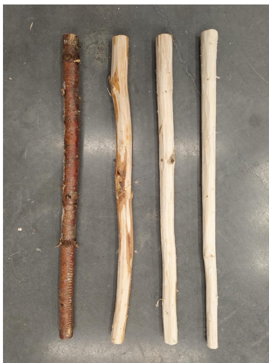
Using a draw knife the spruce bark was removed and material taper exaggerated. On the left a section simply cut from the spruce pole. Moving to the right is the process of coming to the final form prior to sanding.
