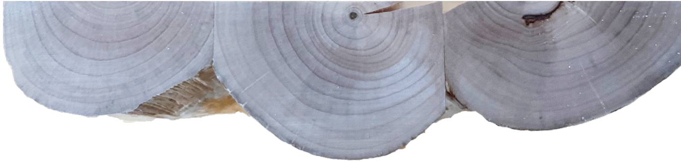
End face of the assembled puncheon floor sample
