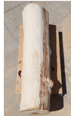
Stripping bark with an angle grinder.
