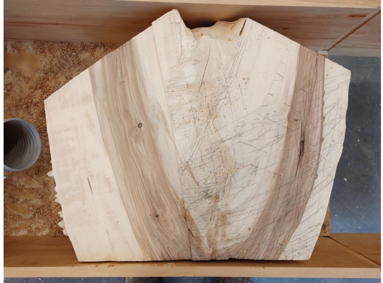
The process of planing: on the right are pencil marks I was using to gauge the amount of material being removed by the electric plane, it was insufficient. The left side is router planed.
