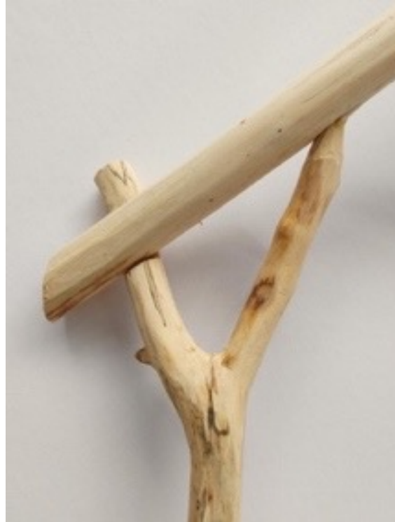
1:10 model of roof and post connection.
