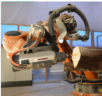
Robotic arm acting as a multi axis CNC machine capable of cutting incredibly precise geometry (Hooke Park 2016).
