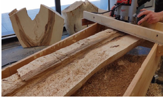
Router planing using the jig constructed with Regan Southcott
