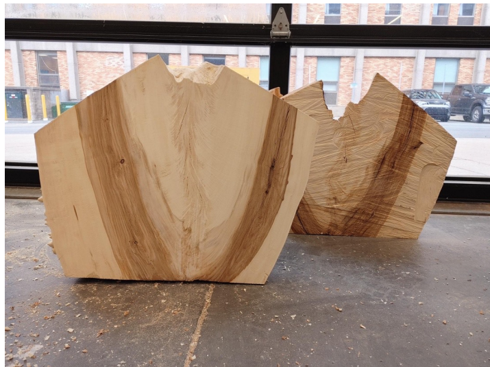
The table tops: foreground is router planed and background is the texture left from the chainsaw cut
