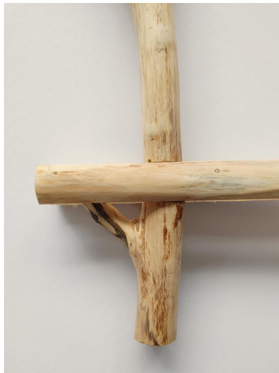
1:10 floor beam and post connection
