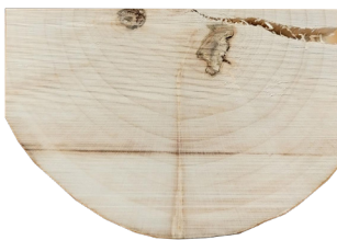
Puncheon. This is a hybrid form milled on three sides simply removing only the required material.
