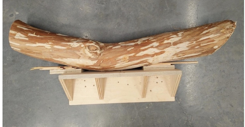
Single curved Pine member fastened to a jig in order to prevent the log from rolling while being cut.
