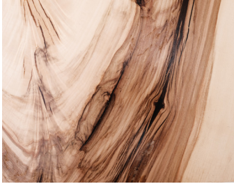
A close up of wood grain in the fork. showing the difference in heart vs crown wood.
