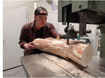
Making the cut. The inside of the curve is being cut using the jig above. Photographed by Regan Southcott.
