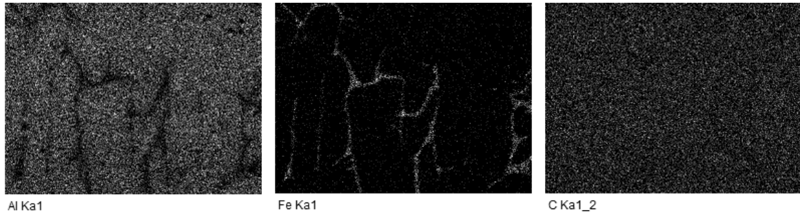
Figure 7-7. EDS mapping analysis for Ti-xAl-yFe for region shown in Figure 7-6
