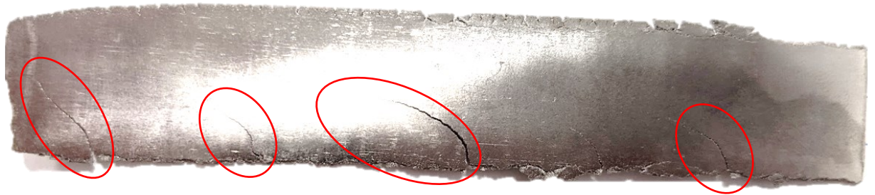
Figure 7-9. Photograph of preferential cracking example on cold rolled samples
