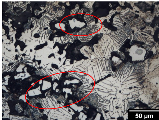
Figure A1. MA particles in a roll compacted Ti-xAl-yV sample sintered for 30 minutes at 1200 °C
