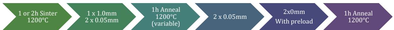
Figure 5-5. Schematic summarizing the rolling path and heat treatments performed on Sample Set 1
