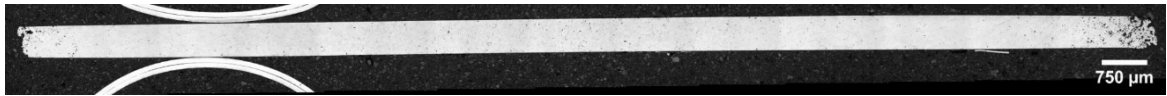
Figure 7-2. Ti-xAl-yFe 1h S+A full strip thickness after the final cold rolling step
