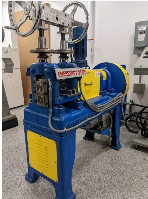
Figure 5-4. Image of the two-high cold rolling mill at Dalhousie University
