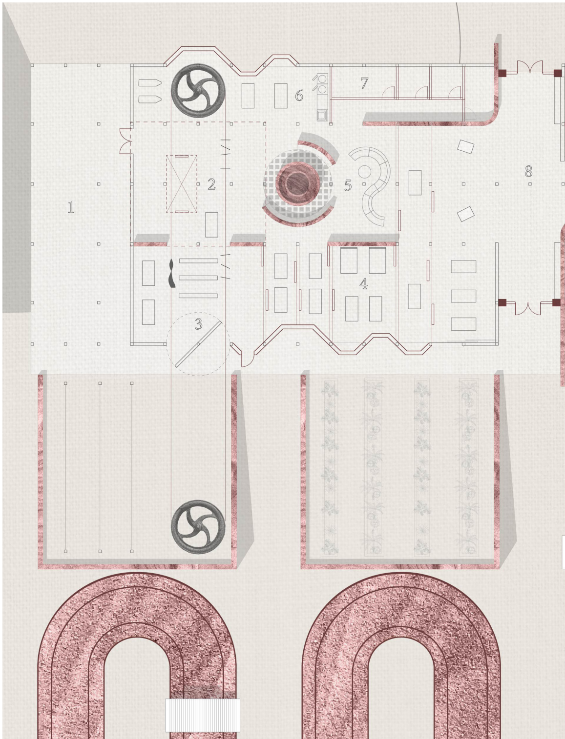
A close-up of the studio plan showing the western textile wing. Moving partitions continue the movement of the clothesline.
