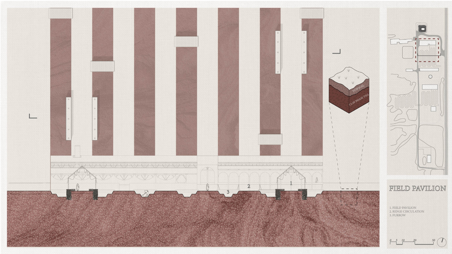
A section of the furrows showing their shaped walls and the field pavilions that are placed.
