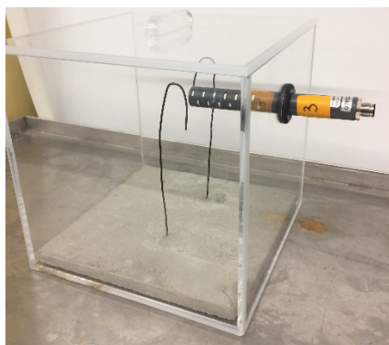
Figure 5. Germination chamber with grout floor and CO 2 probe installed.
