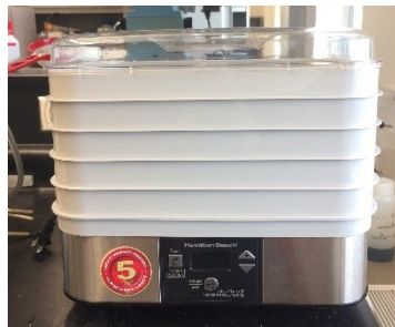
Figure 8. Front view of a benchtop food dehydrator used to kiln malted barley samples
