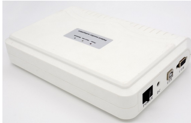
Figure 4.5: The outer case of module PM6750 (240mm x 165mm x 50mm)
