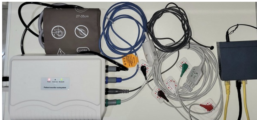
Figure 4.4: Connection of module PM6750 to all medical sensors
