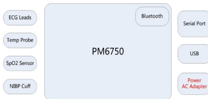
Figure 4.6: PM6750 System Diagrammatic Sketch
