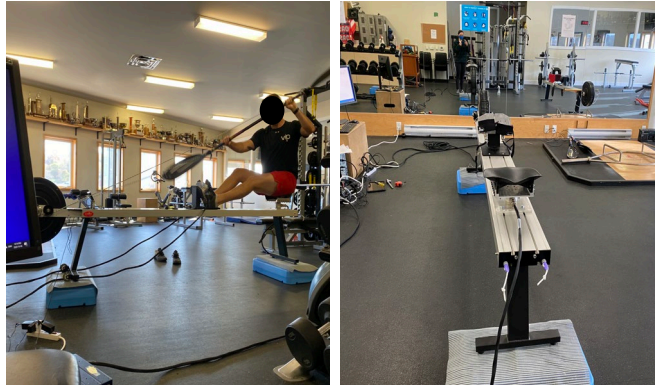
Figure 7. The kayak ergometer set-up and the instrumentation of the three AD2.5D load cells on the kayak ergometer. The ergometer was placed on two boosters to avoid the paddle's blades from hitting the floor.
