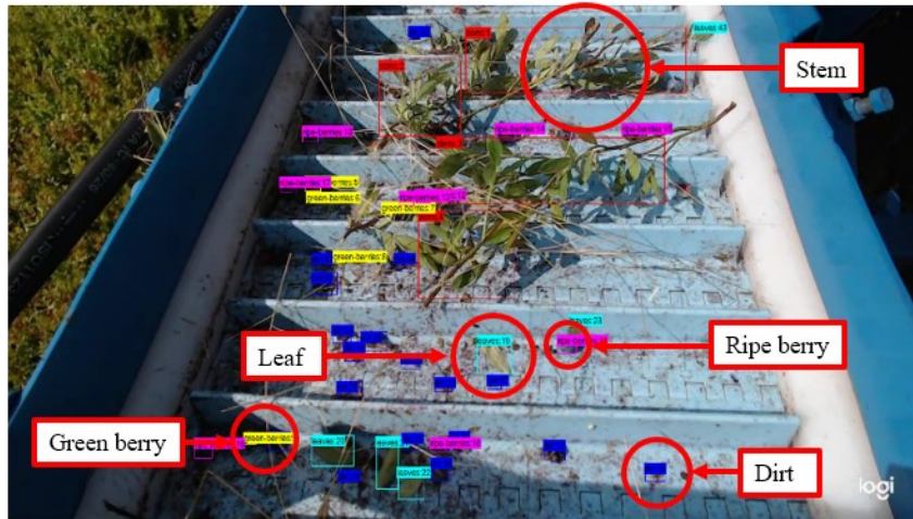
Figure 4-4. Image labeling using custom software developed with the Lazarus compiler
