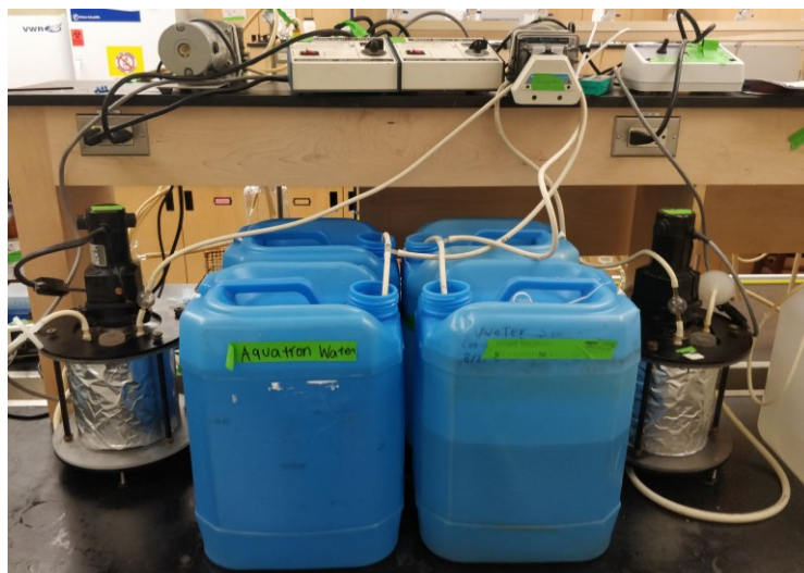
Figure 5.1 Experimental set-up. AR1 (left) tested coupons with GrapheneCoat111 formula. AR2 (right) tested coupons with GrapheneCoat112 formula.
