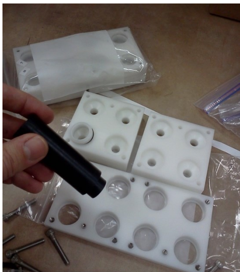
Figure B.5. Foreground: a disassembled SPARTAN cartridge showing the two top 2x2 blocks as well as the bottom 2x8 block.
