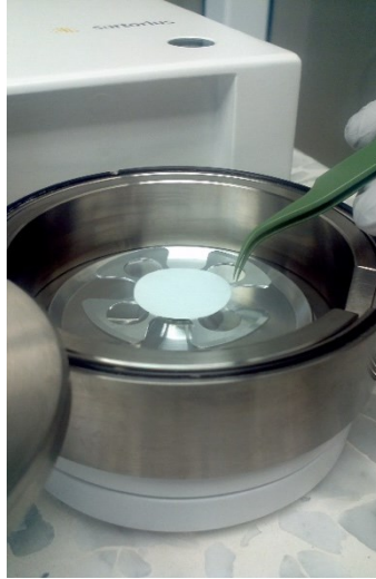
Figure B.2. Example of filter positioned in the center of the balance pedestal
