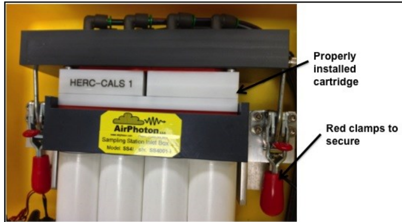
Figure B.17. Example of a properly installed cartridge.
