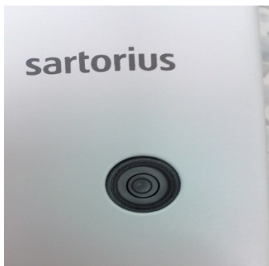
Figure B.1. Indicator bubble on the top of the microbalance. Ensure that the bubble is inside the solid black lines as shown.
