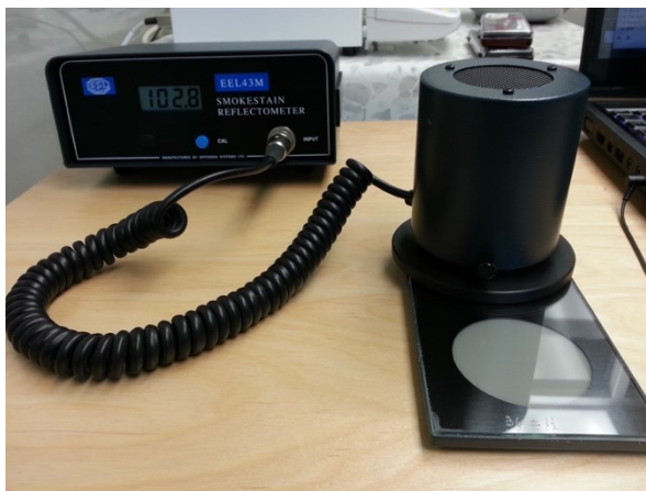
Figure B.7. Smoke Stain Reflectometer, including display, cylindrical optical unit, circular mask, and calibration plate
