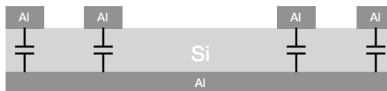
Figure 4.15: Cartoon drawing of capacitive coupling to the ground plane.
