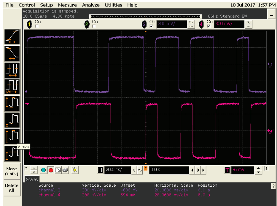
Figure 4.35: Input PRBS sequences used in testing the transmitter.
