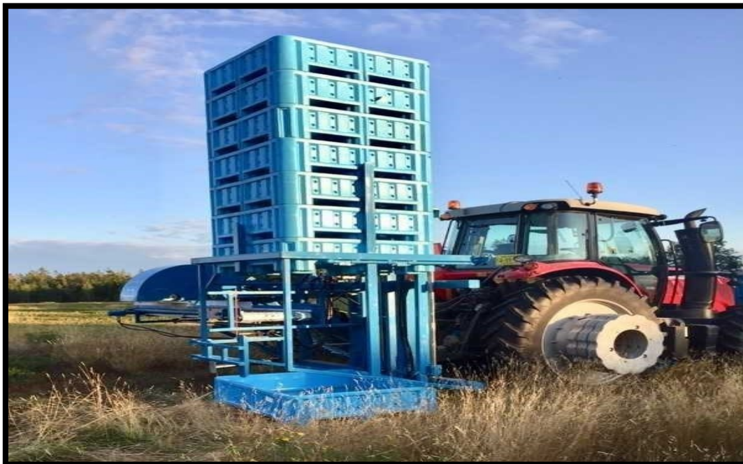
(b) Mechanical harvester with semi-automatic bin handling system.
