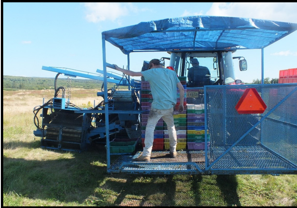
(a) Small box handling system showing manual handling of boxes.
