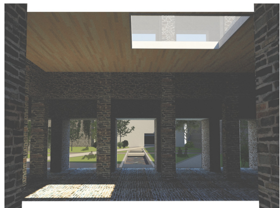
The grotto lies below the southern cloister. In this image you can see the continuous vertical structure through the skylight. The iron stone darkens the room, and a wood ceiling gives the space a warmer feel and absorbs some sound.
