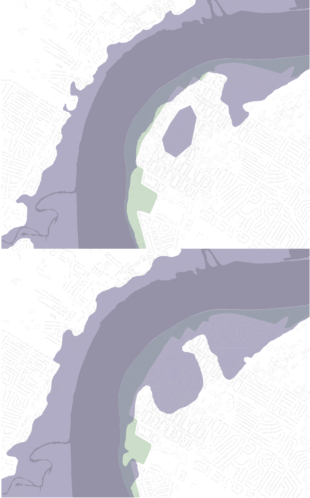
9M (right) and 10M projection of freshet flooding mapped onto Fredericton.
