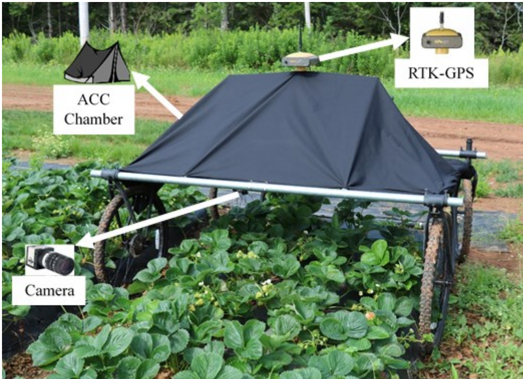
Figure 3-3. Mobile platform for image acquisition in artificial cloud lighting condition (ACC)
