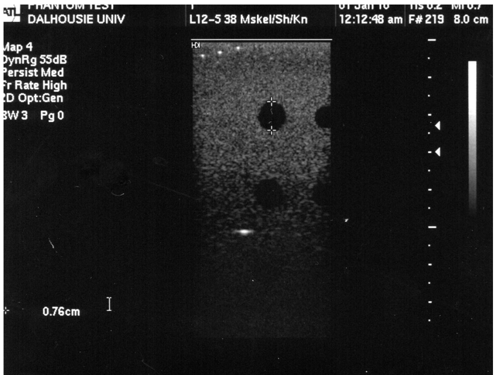
Figure E .2: Ultrasound scan of the axial resolution and hyperechoicity of the US, respectively.
