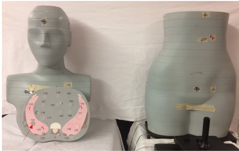
Figure 2.3: Rando phantom with a cylindrical solid water plug (red arrow) to simulate a lung tumor.
