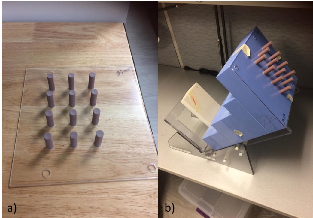
Figure 3.5: The tumor plate with 12 cylindrical tumors (a) and after mounting it to the step phantom (b).
