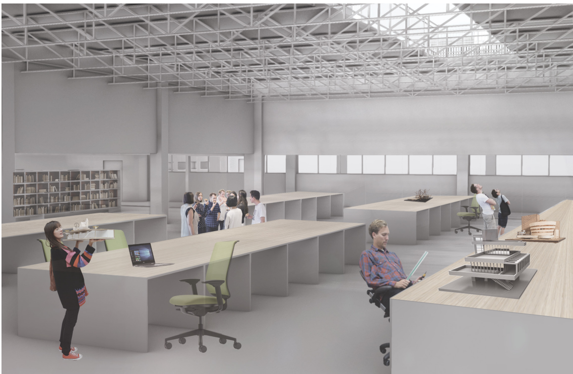
Image 106 The undergraduate studios below receive filtered light from the sawtooth roof through openings in the floor slab
