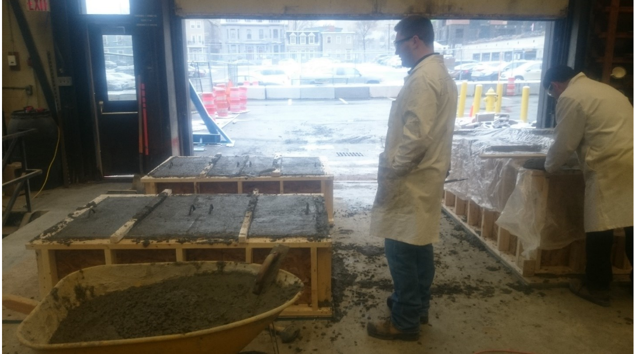
Figure 26: Pouring of the four specimens and end blocks.
