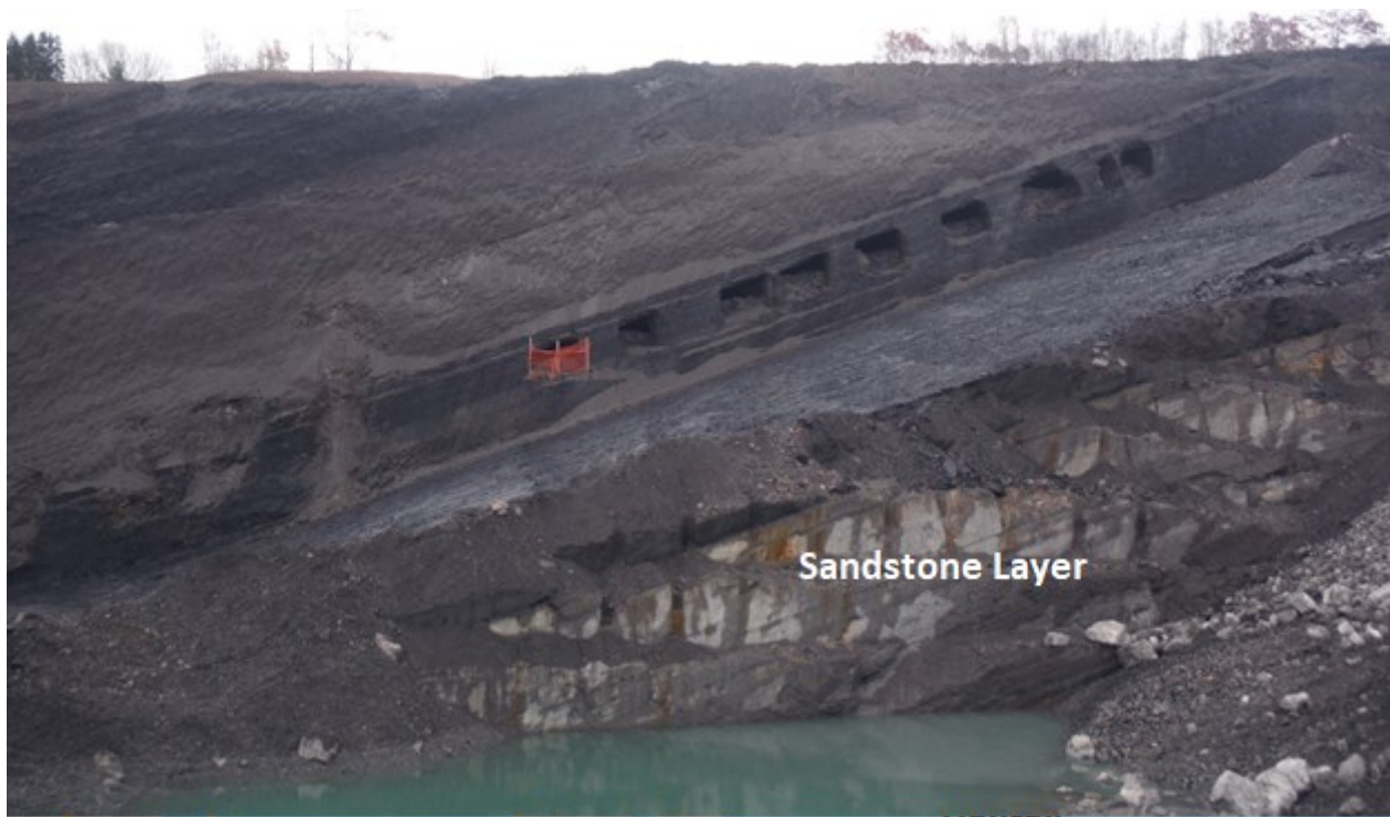
Figure 46: A photo of the side wall of the active open pit the day of testing. Historic underground mining can be seen in the cage seam and the sandstone layer that was to be used to determine the in-situ stress is shown below a layer of coaly shale.
