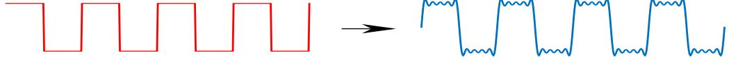
Figure 2.5: Illustration of the idea behind the RCWA. The permittivity profile of the grating (here rectangular) is expanded using the Fourier series. Fourier series are infinite, but we can take only finite number of modes. This causes a the ringing on permittivity profile.
