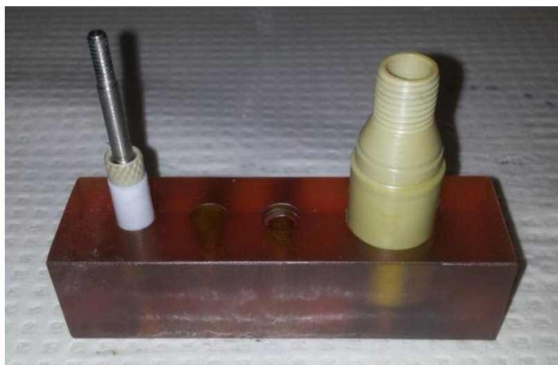
Figure 3.4: A tool designed in-house to help assembly the RDE tip while ensuring the catalyst surface remains pristine.
