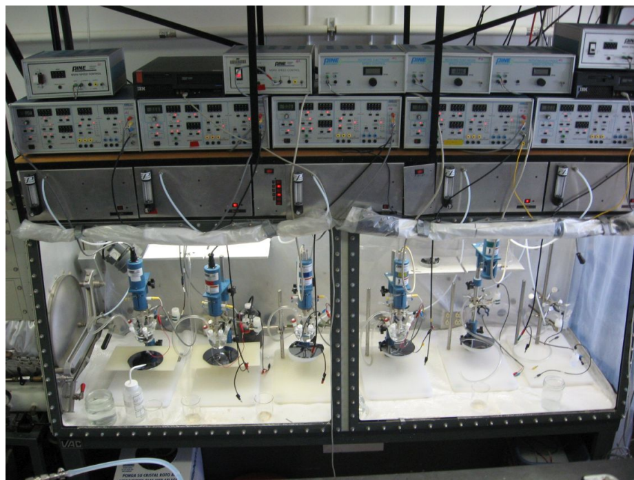
Figure 3.8: Photo of the five RDE stations. (Not all the equipment labelled in Figure 3.7 is shown.)
