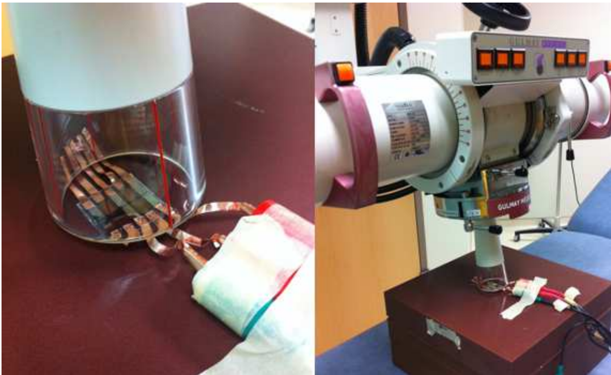
Figure 2.6: Orthovoltage irradiation setup. The substrate consists of 4 OTFTs and the one being measured is aligned to the center of the cone. The OTFT is placed on top of 15 cm of solid water located 30 cm from the source.
