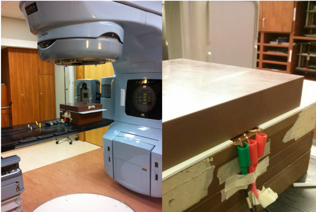
Figure 2.7: MV irradiation setup. The OTFT is placed on top of 10 cm of solid water with 5 cm of solid water on top. To ensure the solid water on top of the OTFT does not damage the device it is propped up with 3 mm shims of PMMA (white in picture) to ensure a small air gap ( \sim 2 mm) between the OTFT and solid water. The OTFT is placed 100 cm from the source with a 5 \times 5 cm 2 field size.
