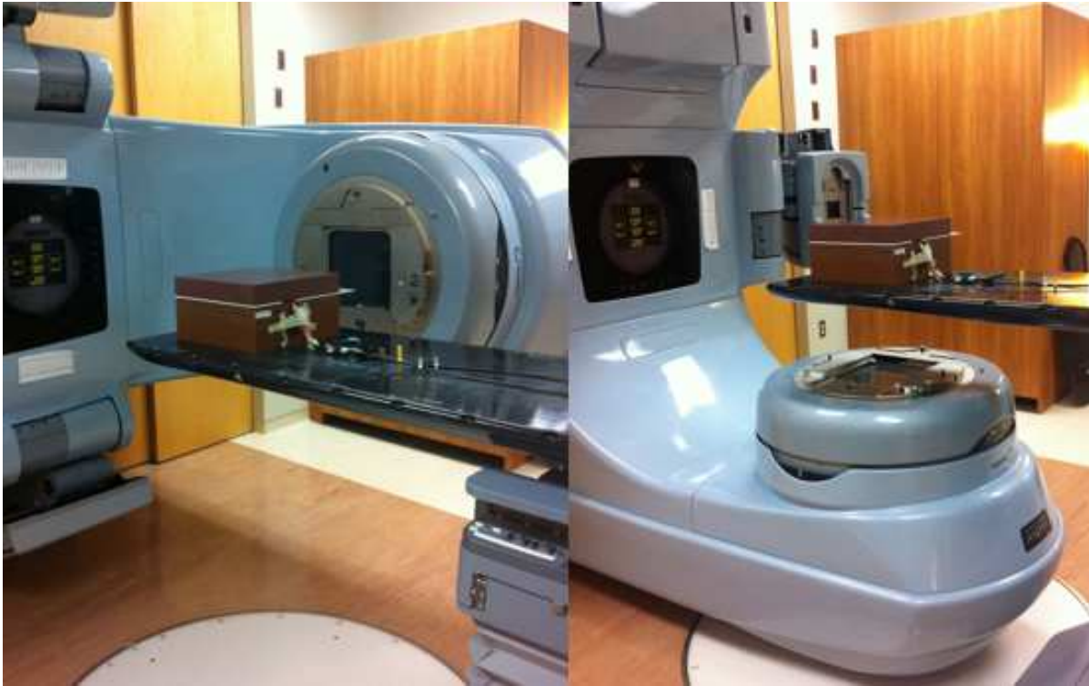
Figure 2.8: Directional dependence measurements. The OTFT was located at isocenter with a field size of 5 \times 5 \text{ cm}^2 . The device was irradiated at 0^\circ (figure 2.7), 90^\circ (left image), and 180^\circ (right image). Ion chamber measurements were performed to ensure equal dose to the OTFT at each angle. During directional dependence irradiations the white PMMA shims were modified so that they did not protrude beyond the solid water (shown in figure) and were made such that the device was at a depth of 10 cm when irradiated at 90^\circ .
