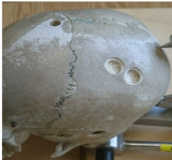
Figure 5.21 Drilling Tests on Human Skull using PA10 Robotic Manipulator
