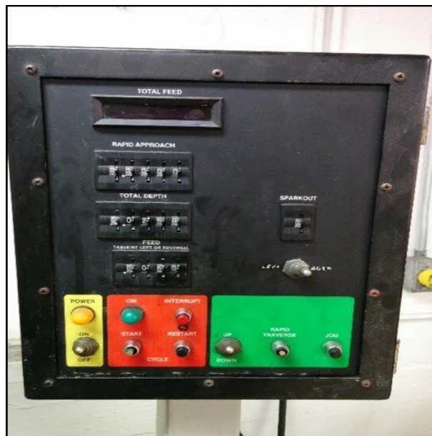
Figure 3.10 Top right panel of the grinding machine (Photo courtesy of J Perrier-Daigle).
