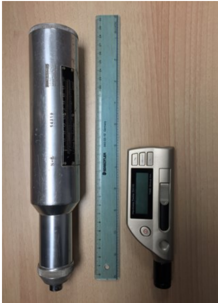
Figure 2.6 Leeb hardness tester vs. Schmidt hammer
