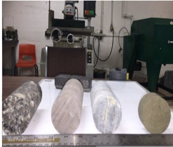
Figure 4 Core specimens of sandstone, granite, dolostone, and schist were selected to evaluate the number of impacts required to validate a test
