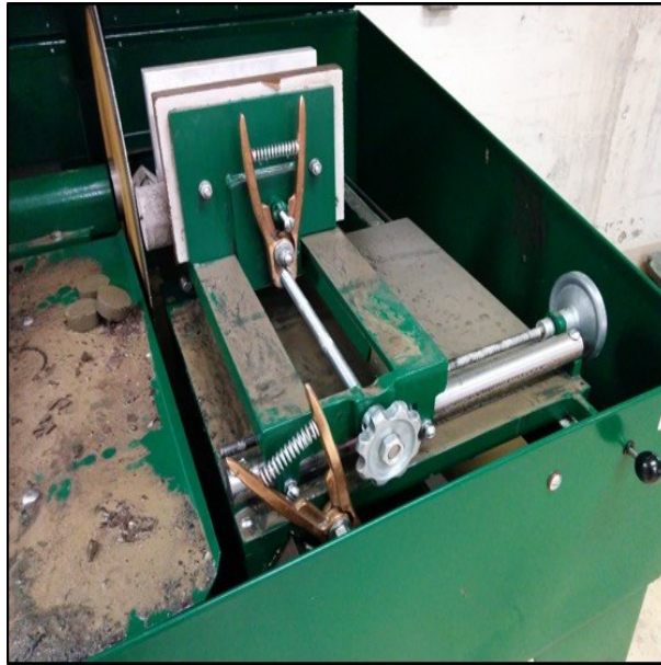
Figure 3.5. Close up of vice controls inside the wet blade saw machine ("Photo courtesy of J Perrier-Daigle).
