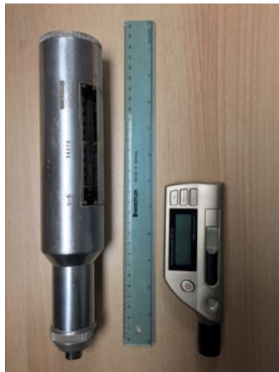
Figure 5.9 Comparison between Leeb hardness tester (LHT) and Schmidt hammer, type R
