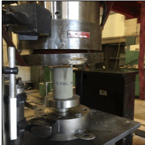
Figure 3.12 UCS test machine with a sandstone sample.
