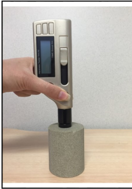
Figure 1. Leeb Hardness Tester. The lightweight and compact size of the device make it convenient for fieldwork.
