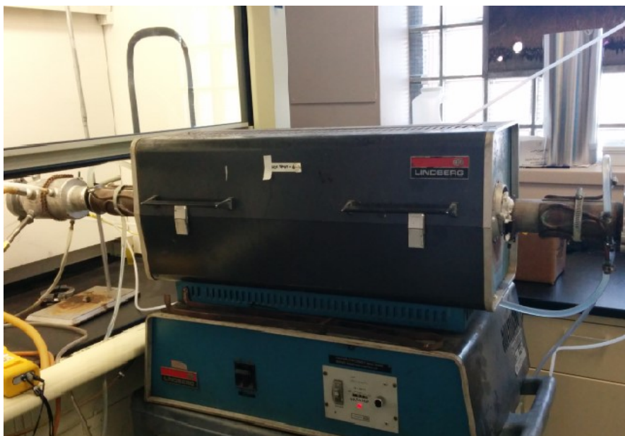
Figure 8. Lindberg electric tube furnace for bench-scale emission experiments.
