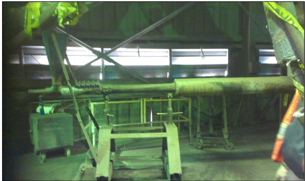
Figure 36. Separate burner pipe constructed to be used for shingle delivery into kiln.
