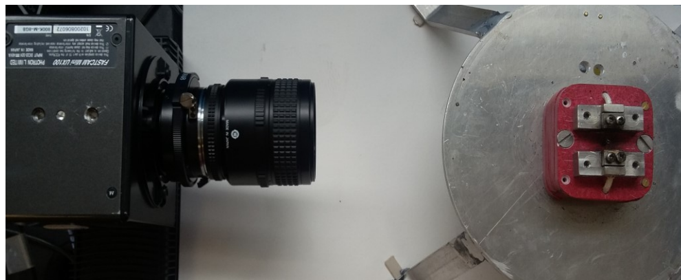
Figure 23. Camera-Heated Grid Reactor set-up for fuel blend ignition study.
