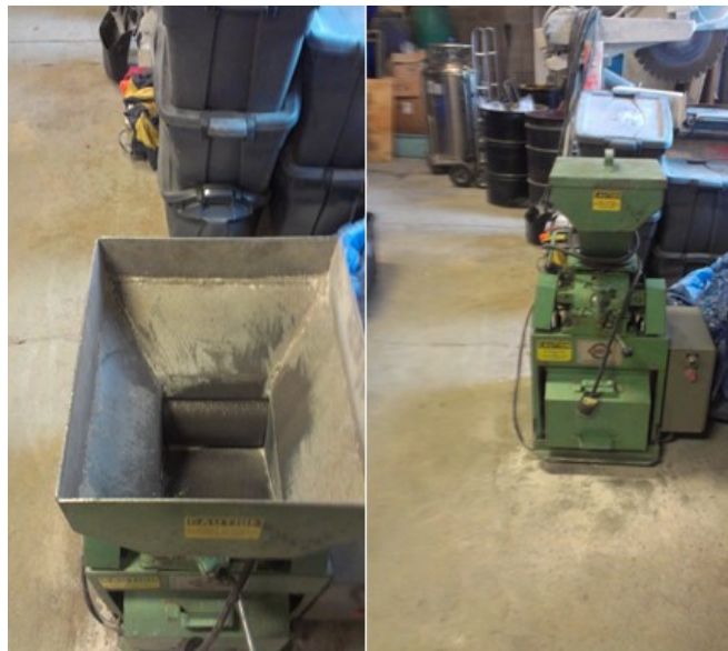
Figure 11. Hammer mill crusher used at Dalhousie University.
