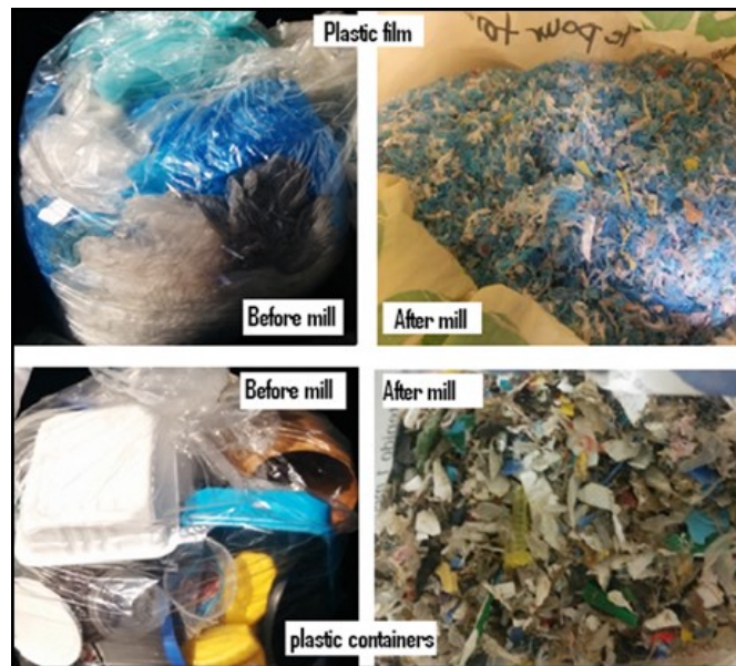
Figure 12. A selection of received plastic based waste (plastic film and plastic containers) before and after size reduction.
