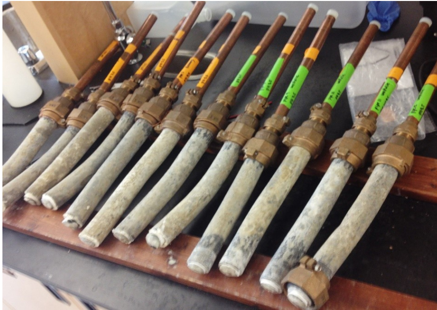
Figure 3.2.3: Harvested pipe sections undergoing treatment
