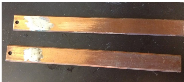
Figure 4.2.2: Coupons with 50:50 lead tin solder prior to corrosion
