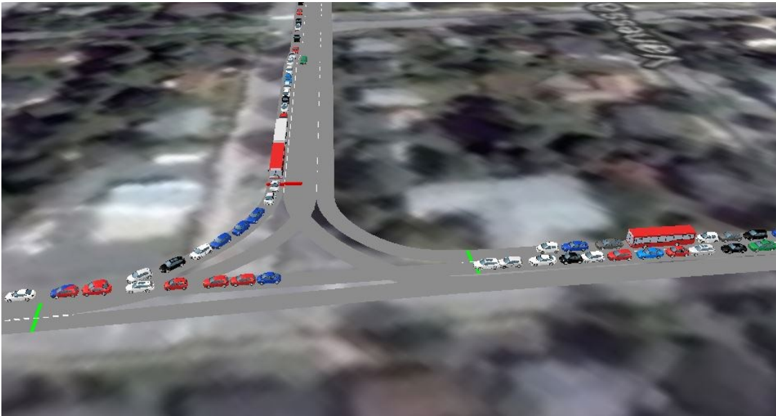
Figure 4-7 Queue Build Up in Traffic Microsimulation Network Model
