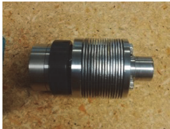
Figure 3.9. Fifteen thou disk pack spacing, with magnet and bearing.
