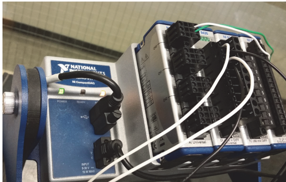
Figure 3.20. DAQ chassis with corresponding modules.
