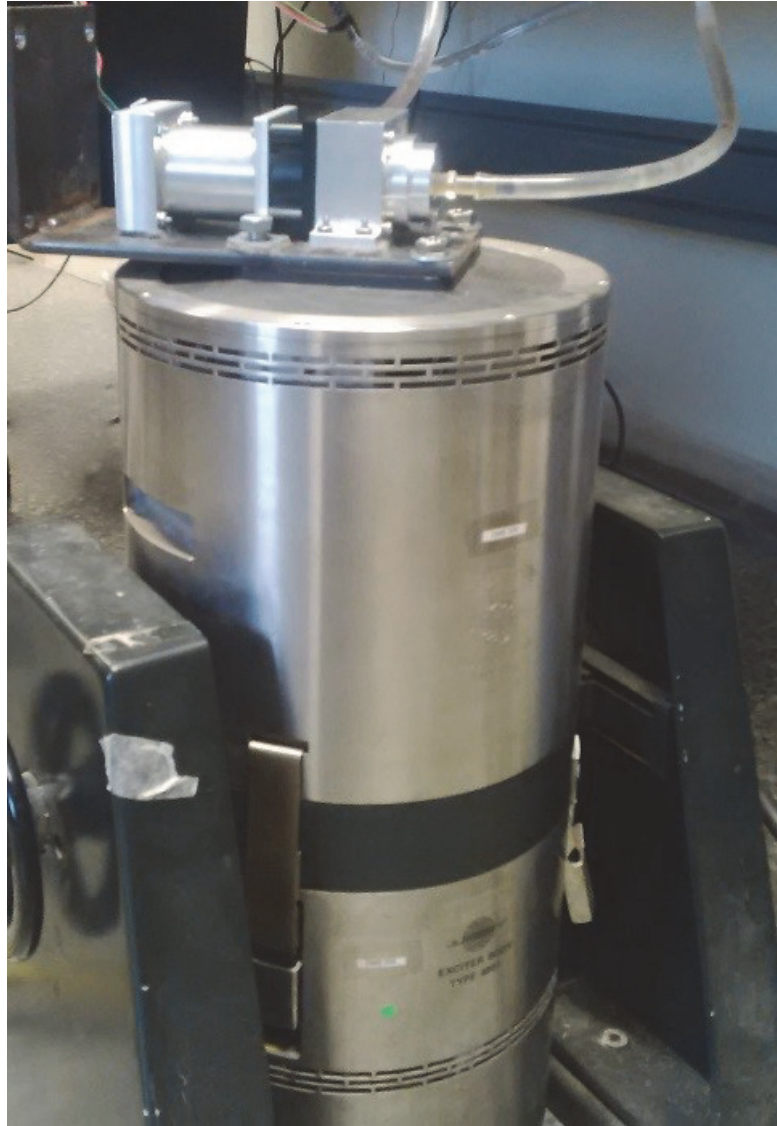
Figure 3.19. Prototype pump on the Vibration Exciter System i.e. shaker table.
