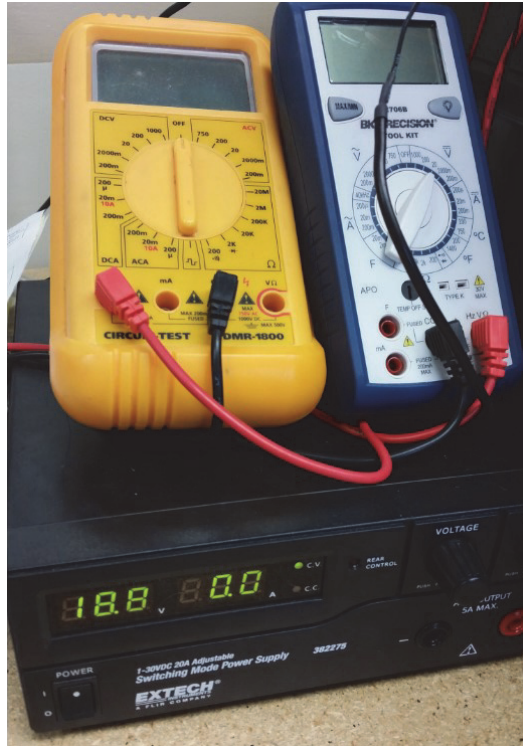
Figure 3.17. Power supply used for motor control, and multimeters.
