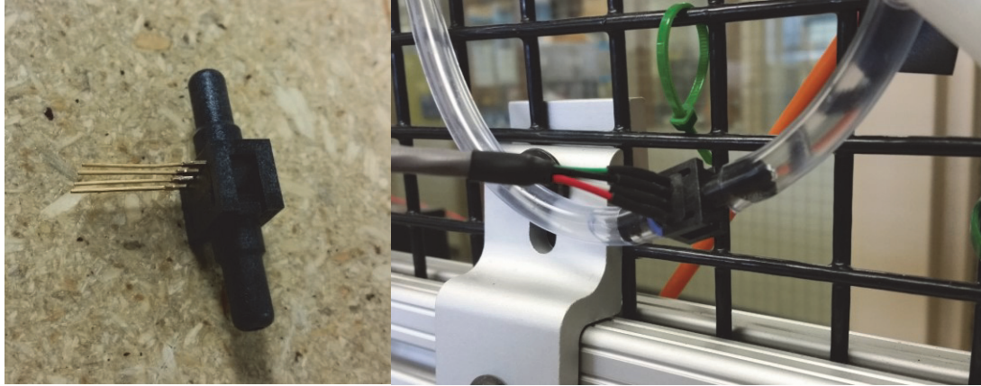
Figure 3.14. Differential pressure sensor, PX-26 meter unwired (left), and the pressure sensor in the set up (right).
