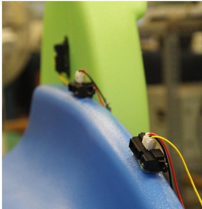
*Figure 6: Sharp Sensors attached to Slide*
