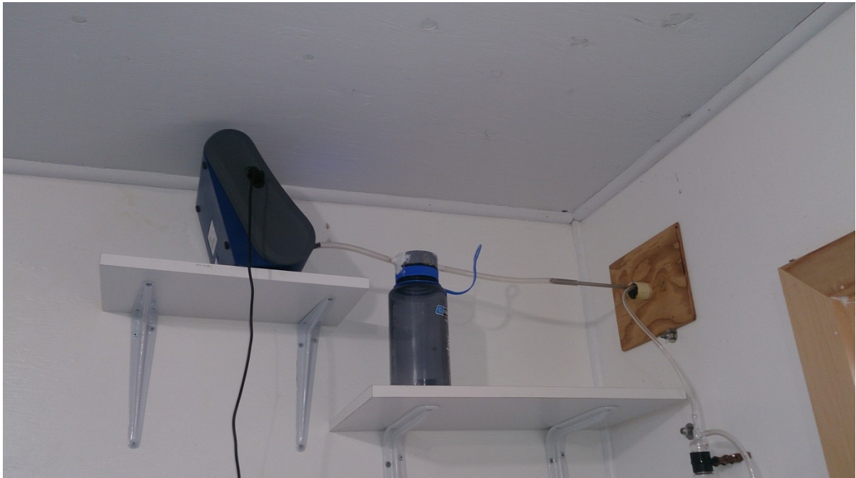
Figure 11. TSI DustTrak DRX Aerosol Monitor model 8533 and water trap on Sable Island (Barnett, 2016)
