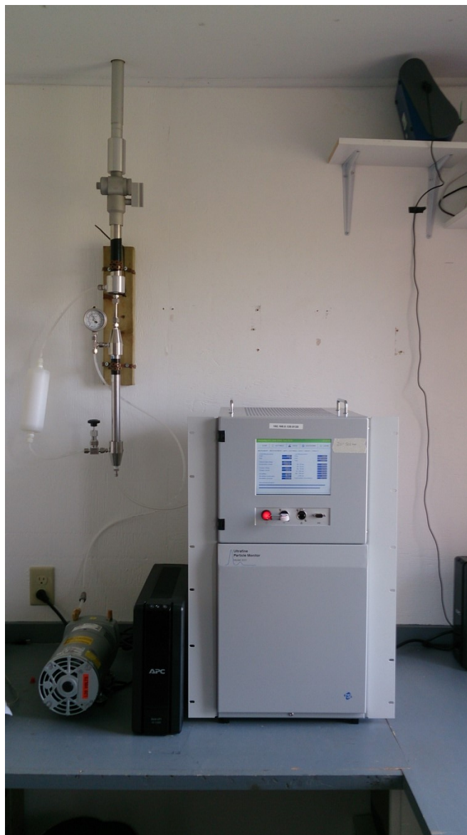
Figure 15. TSI Ultrafine Particle Monitor model 3031 and TSI 3031200 Environmental Sampling system on Sable Island (Barnett, 2015).
