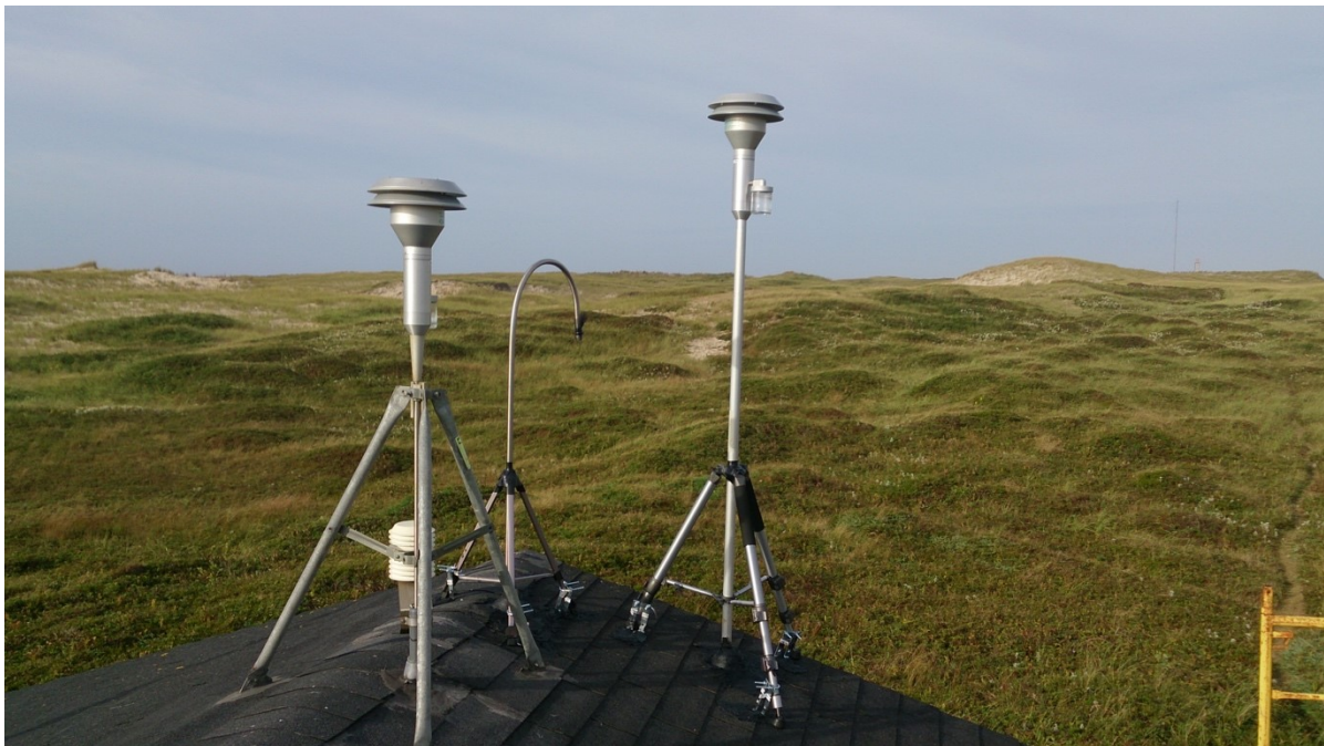
Figure 7. Existing (left) and new sampling inlets (center, right) installed on Sable Island air chemistry shed (Barnett, 2015)
