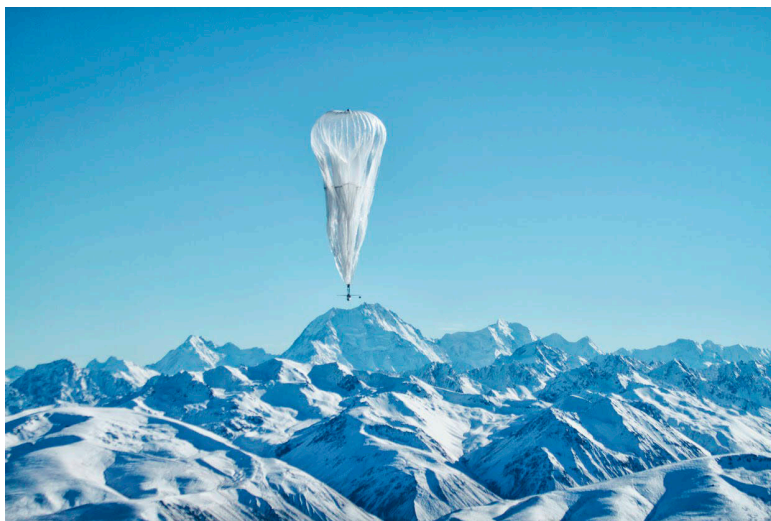
Google X's "Project Loon" distributes the Internet via balloons that use wind currents in the atmosphere to float to destinations around the southern hemisphere, namely "last-mile" destinations that are the most difficult for network infrastructure to reach; image from Google Project Loon.
