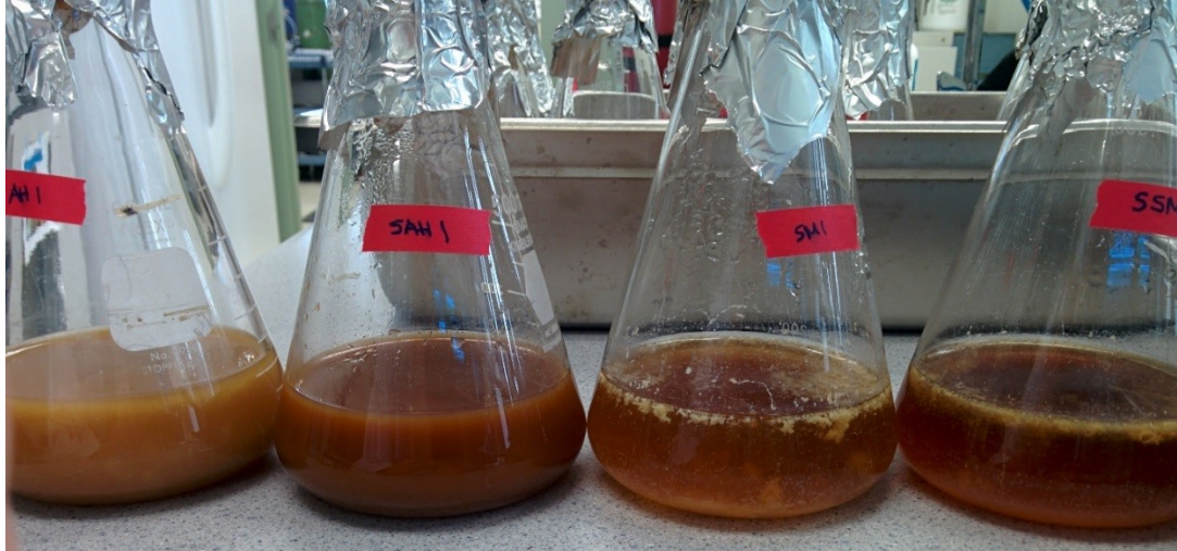
Figure 4.1 Observation of the color change and precipitate formation in the experimental flasks for 2015-500ML-01 of the raw hydrolysate, supplemented hydrolysate, spent media, and supplemented spent media (left to right).
