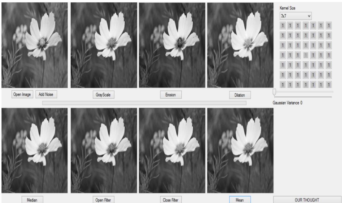
Figure 45: Snapshot of the C# morphological operations platform. The top left-hand image is the original image, followed by the grey-scale image. The subsequent images show the effects of using filters.
