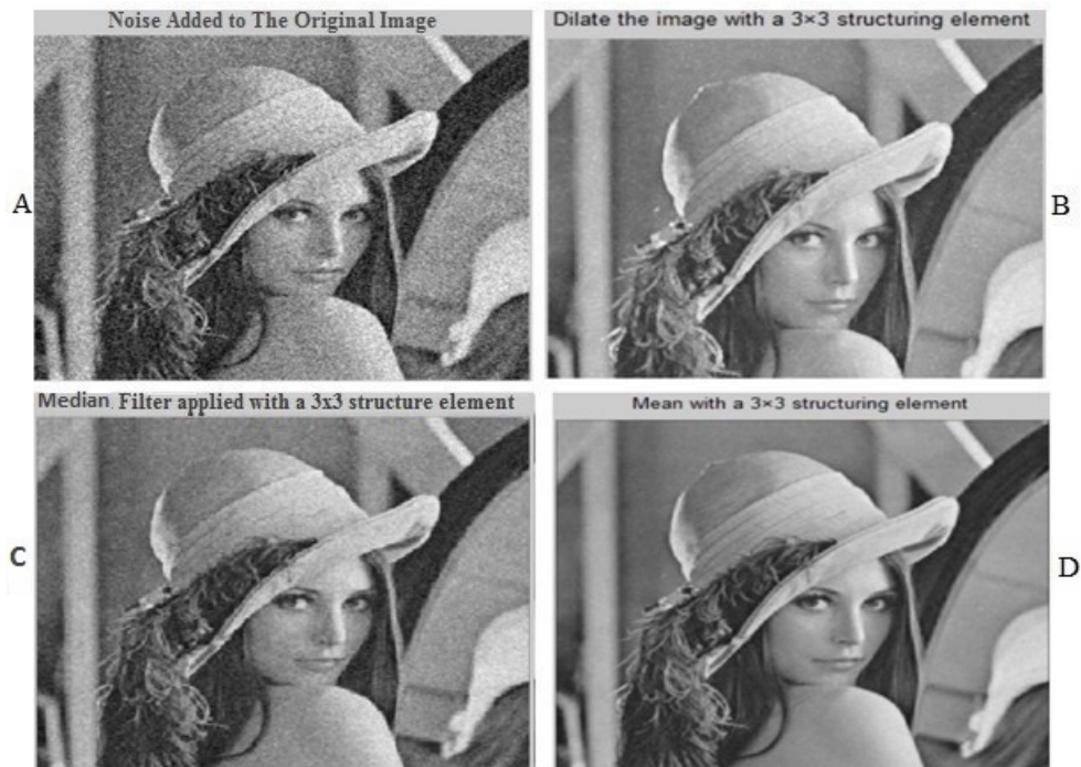
Figure 40: Illustration of the effect of applying dilation, mean and median filters with a 3 \times 3 square structuring element. Images B, C and D show the effect of using a dilation, median and mean filter, respectively.
