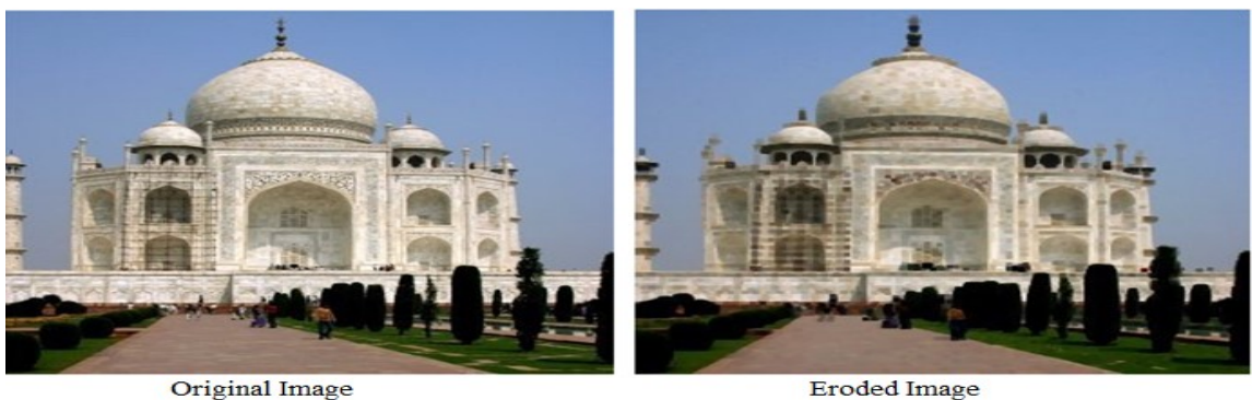
Figure 17: The effect of using an erosion filter on a colour image.
