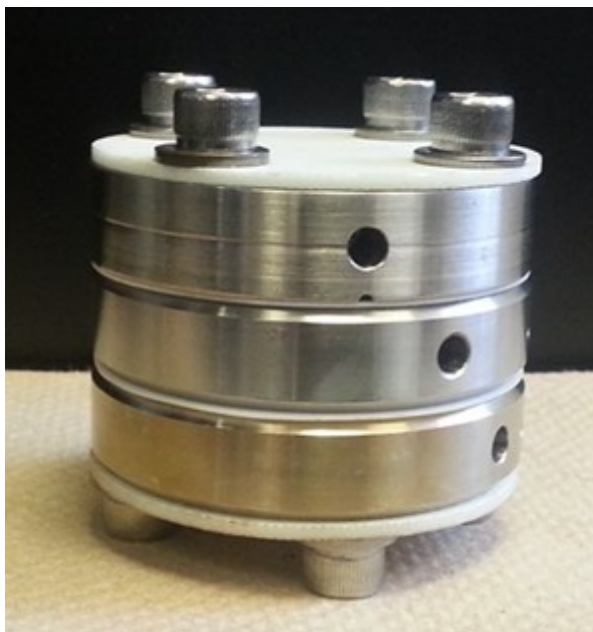
Figure 4.6 (b): A photograph of a fully assembled 3-electrode Conflat cell.
