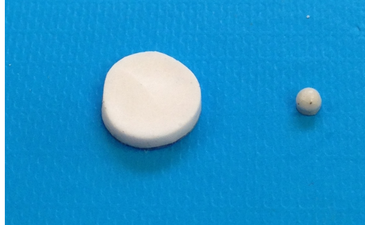
Figure 15: Digital image of a G2 axial pressed disk and a G2 CIP processed pellet.
