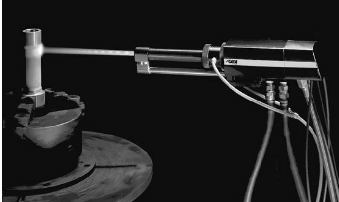
Figure 16. HVOF in operation.[96]
