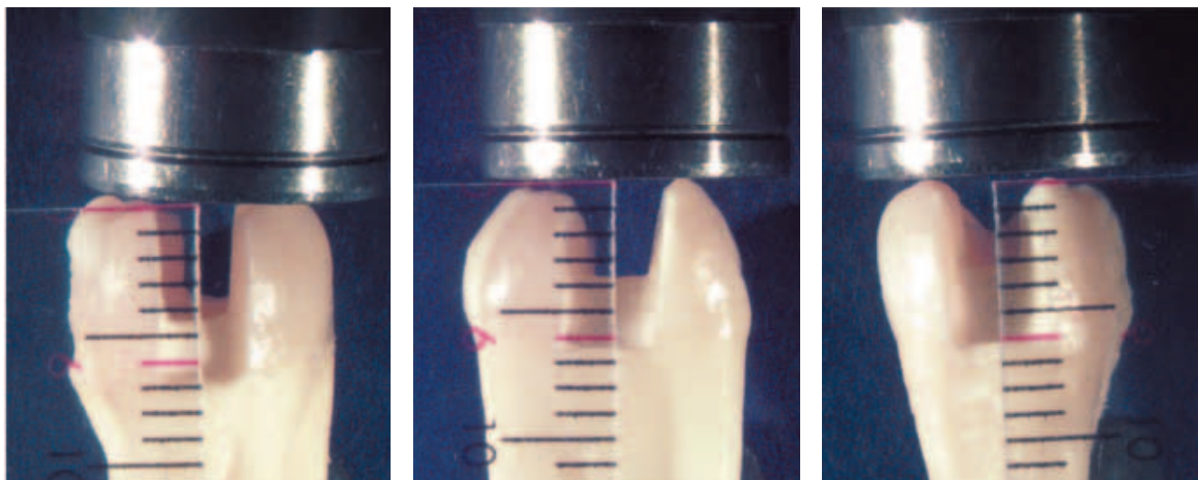
Fig 1 Three tooth preparations extending just past the cemento-enamel junction showing a preparation floor-to-light-guide distance of (left to right) 6.9 mm, 6.5 mm, and 6.2 mm.
