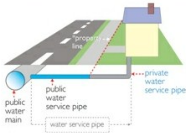
Figure 2.4: Schematic diagram of typical residential water service (DC Water and Sewer Authority, 2012).
